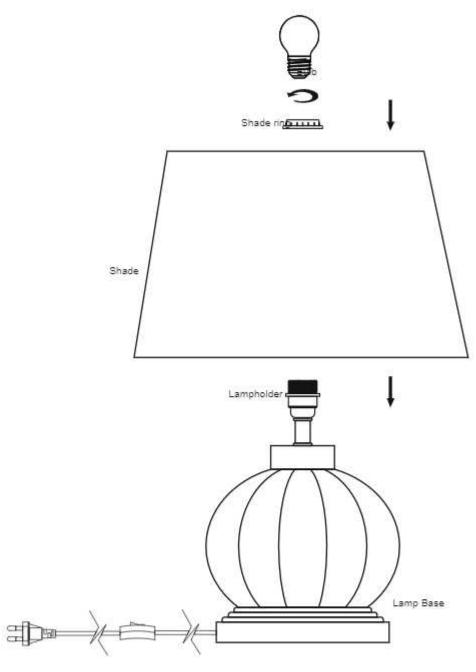
Being with the base by placing it upright on a flat, even floor surface.
